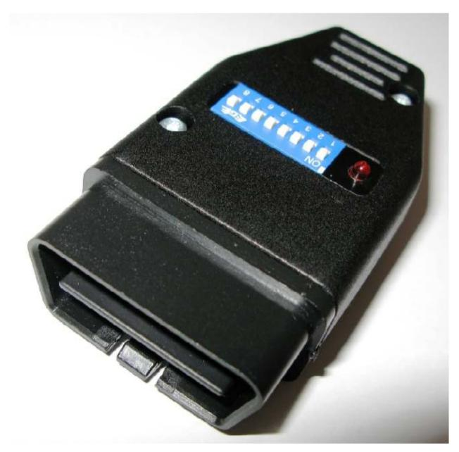
To activate bypass functionality of device switch number 8 should be ON.
