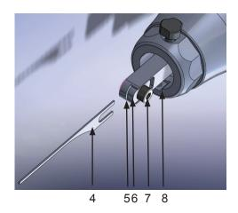
Open the clamp screw (7) with the included Allen key. Place the pick needle (4) into the resulting gap (5) between holder (8) and clamp (6) and push the pick needle all the way to the stop. Tighten the clamp screw (7) with the Allen key so that a firm hold of the needle is ensured.
