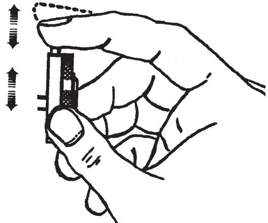
Insert the tension tool TNT-20 into the keyway.
