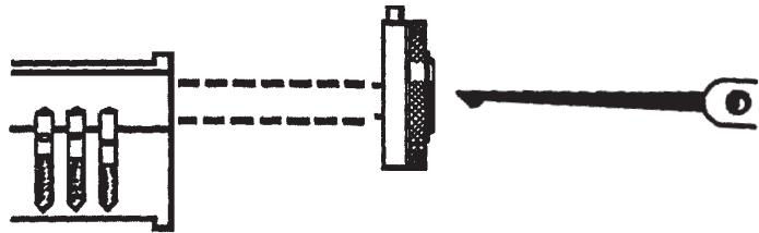
With the tension tool TNT-20 you exert a slight tension to the plug in the wanted direction.
