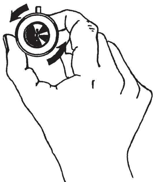
The tension tool TNT-20 disposes of two pins. These pins have to be inserted into the cylinders keyway.
